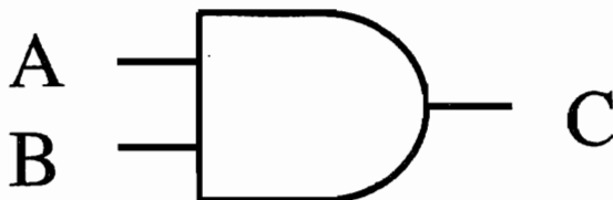
Fig. 5.9 The AND Gate
